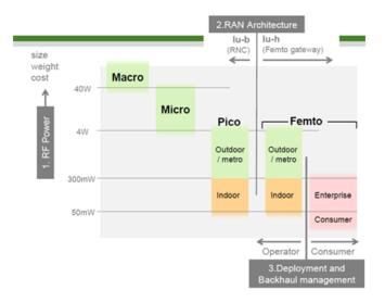
Figure 1: Small Cell Types and Characteristics (Source: NGMN)
