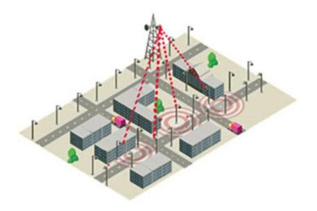
Figure 5: Sub 6 GHz Point-to-Multipoint Backhaul Links
